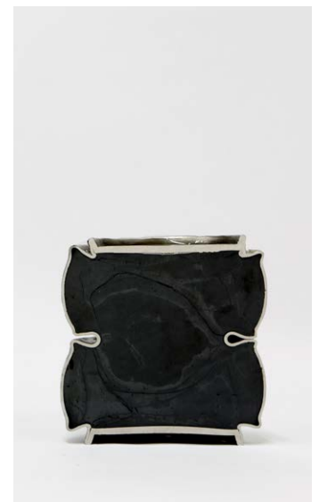
Synroc can and cut-away of the synroc wasteform.
